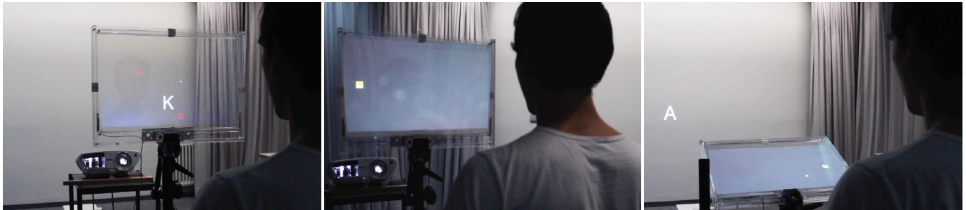
Figure 1. We conducted an experiment comparing a transparent display (left) with typical display configurations such as a conventional display at an angle of 30° (center), and a horizontal display (right) in a dual-task scenario (square-click as primary task, background observation as secondary task). Results show constant primary task performance for all configurations, but an increase in background awareness (i. e. stimuli detection rate) for the transparent (83%) and horizontal (70%) display.
