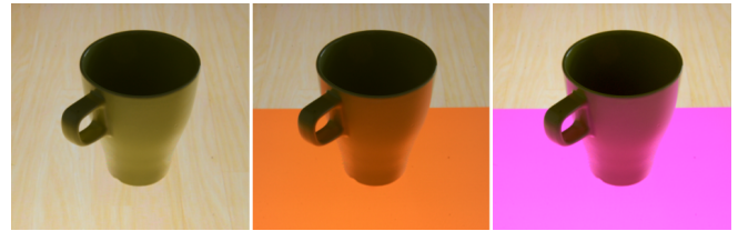
Figure 8. Effect of color with an reflective opaque surface. The reflection on the surface in combination with the displayed color alter the target's color.
